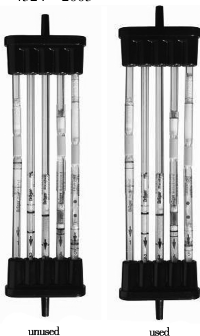
Fig. 2 Simultaneous Tests Set Container Aeration I (81 03 380)
